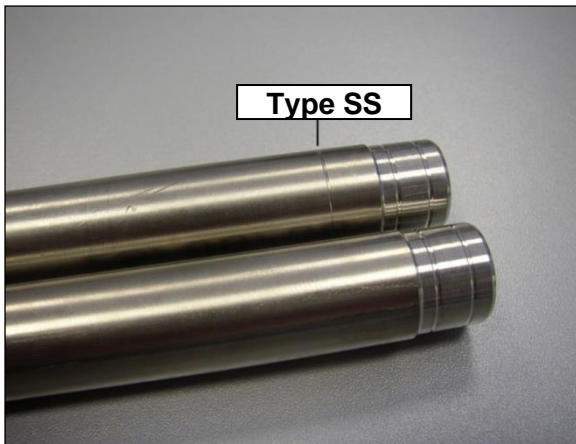
Figure 3 Notch to differentiate the two cartridge types
